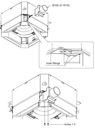
\* When using the "UTZ-KXGC" kit for high humidity, please first cut off and remove the heat insulation as shown in the figure.
