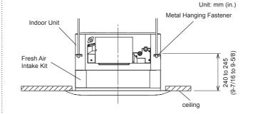
Attach the Fresh Air Intake Kit to the main body using the bolts provided
